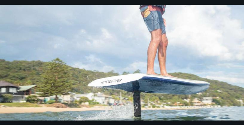
The HydroFlyer<sup>™</sup> uses a bluetooth controller attached to the handlebars to control the speed. The controller feeds the signal to the onboard computer, which in turn signals the lithium battery to power on the silent motor. Once the rider reaches a speed of around 3-4 knots, the power of lift and thrust begin to work its magic and the hydrofoil comes out of the water.
